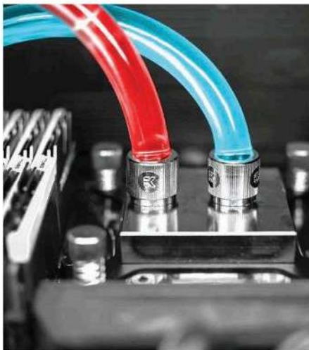
Cold Plate (Chip Level Cooling)
