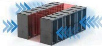
Hot aisle containment
